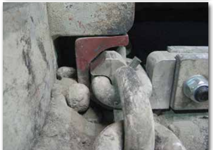
Universal push-fit flight holders give operators the option of re-using existing flight bars and running long-strand chain assemblies
