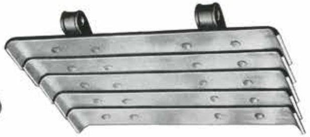
The conveying surface is composed of steel plates (top view)
