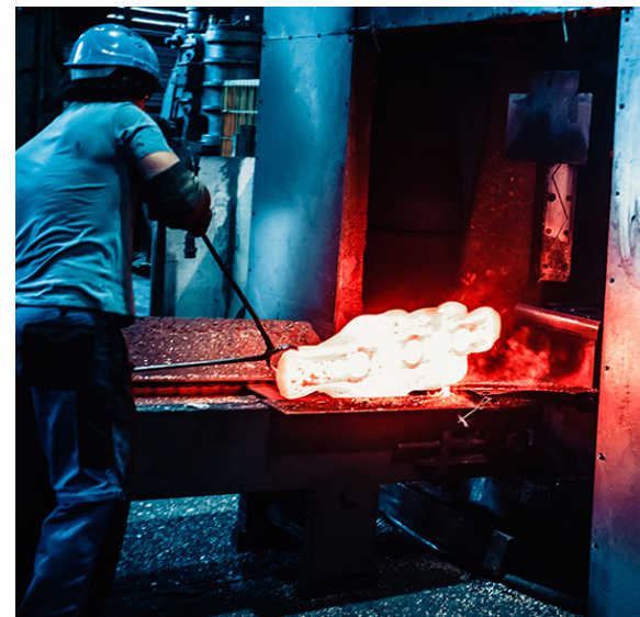
Square billets (edge length 50 to 120 mm) or round stock (18.5 to 200 mm in diameter) can be used as feedstock material.
